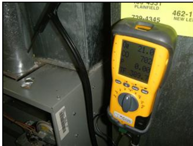
8.0 Picture 2 CO - 702 ppm at Steady State
